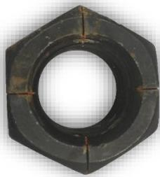
Figure 11 Surface Discontinuities Test Sample
