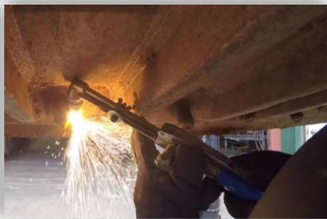
Figure 2 Cutting Edge Blade Replacement
