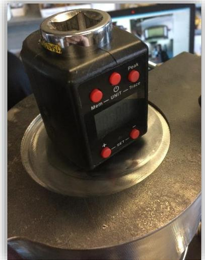
Figure 21 Torque Sensor
