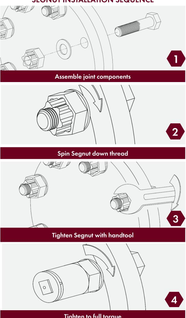
Tighten to full torque
